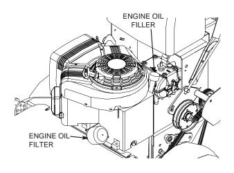
Figure 7-1. Briggs & Stratton Engine Oil Fill/Dipstick, Filter and Drain Locations
